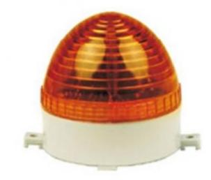
High-performance xenon lamp as the light source strobe warning lights; unique flash type shade, so better visibility light signal; Material: shade -PC, base -ABS; product structure compact, flexible and easy fixed; flash frequency: 90-150 beats / min; protection IP54
