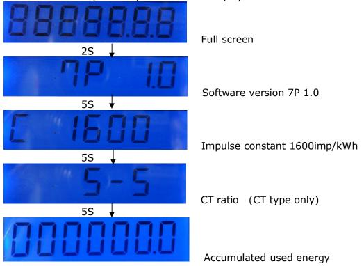
If the CT ratio is less than 150:5, the LCD display will shows 6 integrals plus 1 decimal. If the CT ratio is set bigger than 150:5, then the LCD will show 7 integrals.
